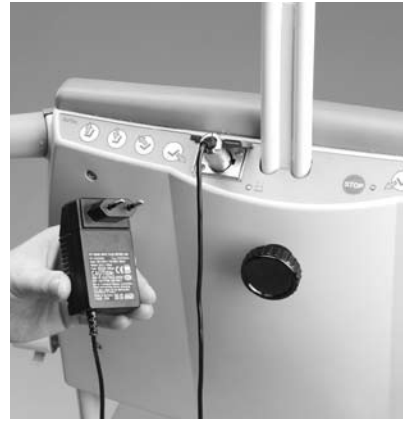
Charger connection point
