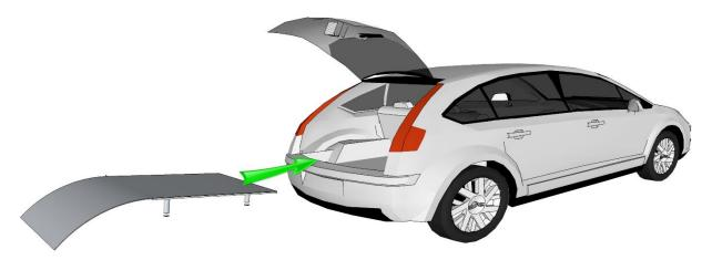
Place Easy Loading on the guard plate and attach the capstans.
