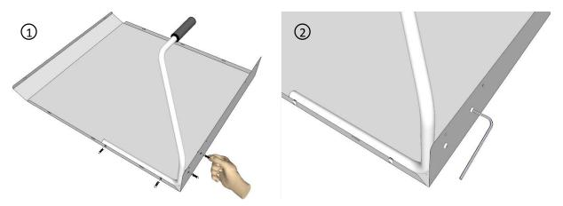
Screw the two smaller handles in Easy Loading lifting plate, 4 screws. See Figure 3-4.
