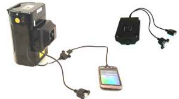
LIPO-USB-CONNECTION-HOUSING FOR THE BATTERY TO CHARGE ALL COMMON USB-DEVICES
