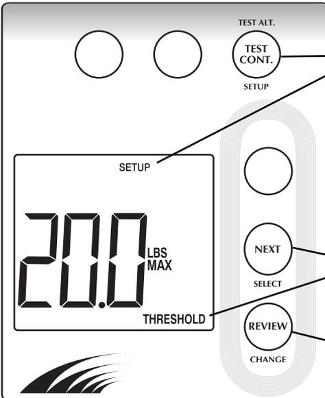
*Press this button until console is in “Setup” mode. After parameters are set, use this button to exit back to “Test” mode.*
