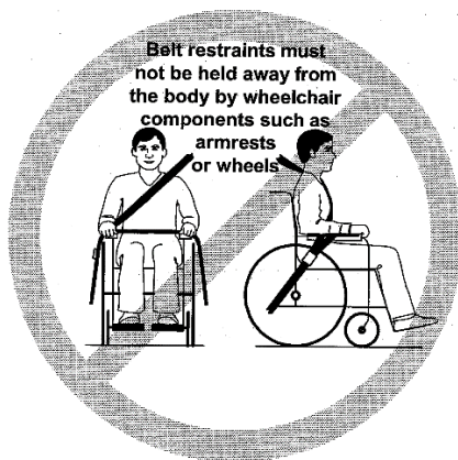
Figure 6 — Illustration of improper belt-restraint fit
