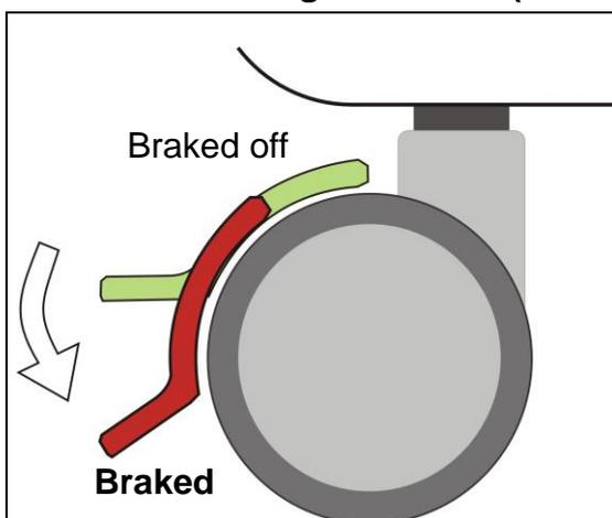
Bedside cabinet ELEGANZA CLASSIC is equipped with 4 castors, of whom 2 or 4 are individually braked (acc. to model number). The way of braking or braking off is shown on the picture.
