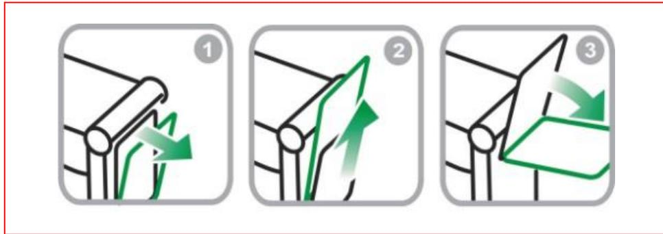
1. Pulling the handle in arrow direction (fig.1) tilt the desk out of a table body.
