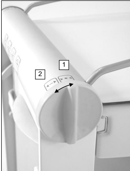
Turning the handle to position 1 the table brakes are activated.
