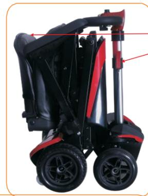
1.Use one hand to hold the steering column, other hand hold the back of the seat.
