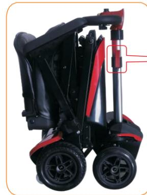
Use your right hand and squeeze the release switch toward the silver steering column. Do NOT pull red lever.
