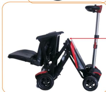
Press the footboard downward to completely open.
