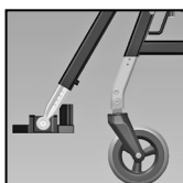
T2-D: 2 holes visible
