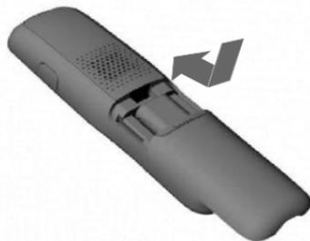
2. Align the cover flat against the battery compartment, and then slide it upwards until it clicks into place.
