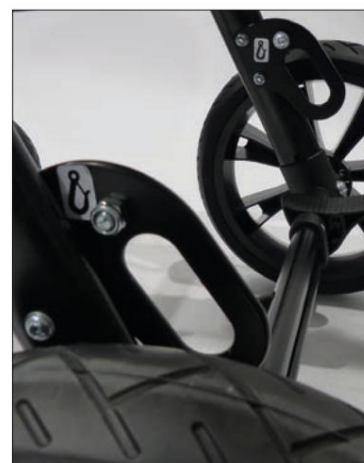
Attachment points, rear according to ISO 7176-19
