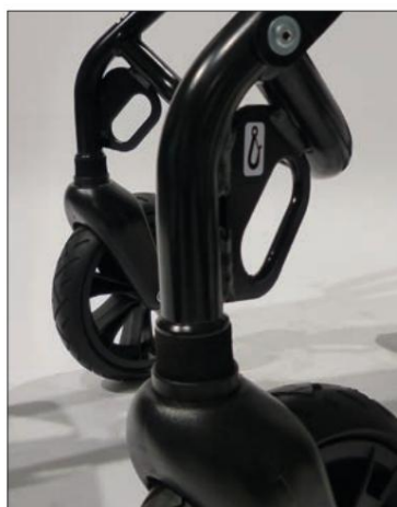
Attachment points, front according to ISO 7176-19
