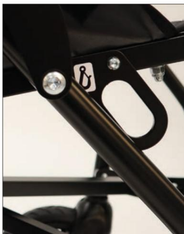
Attachment points, front according to ISO 7176-19
