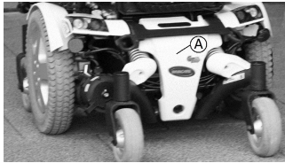
Power module behind rear shroud A Fig. 6-2
