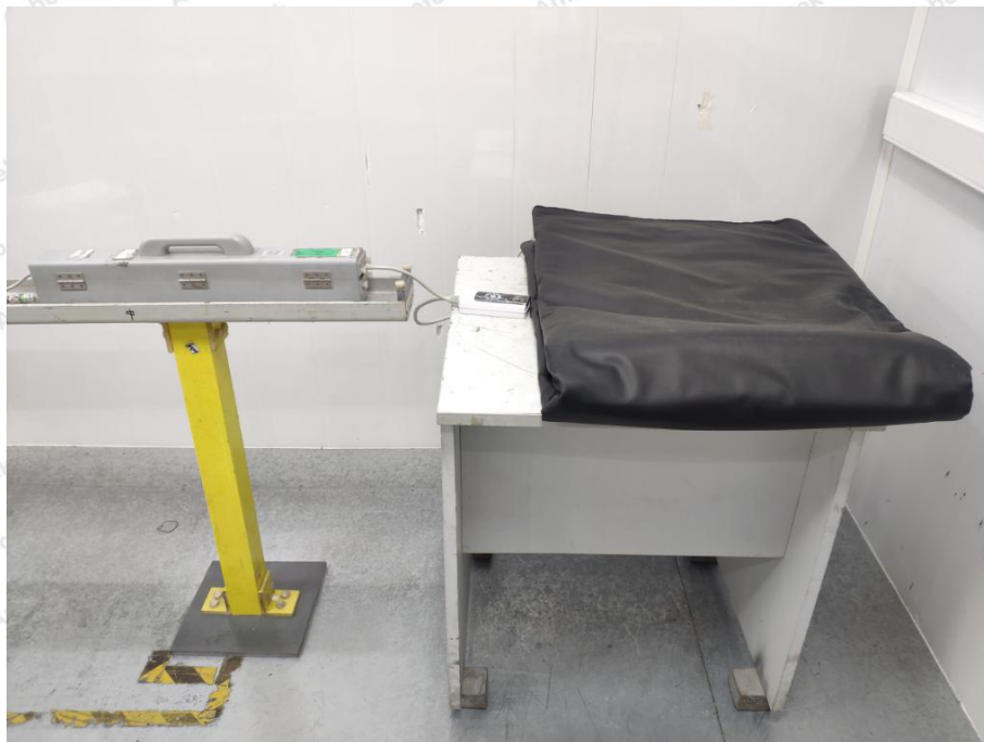
Photo of Disturbance Power Test
