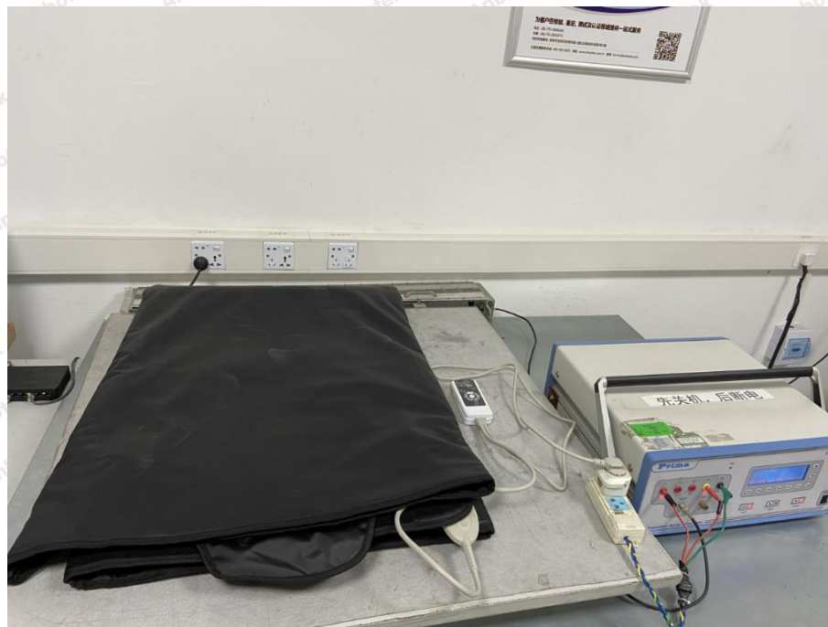
Photo of Electrical Fast Transient/Burst Immunity Test
