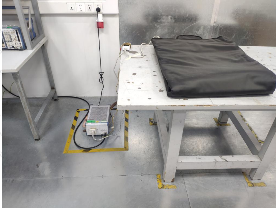
Photo of Power Line Conducted Emission Test
