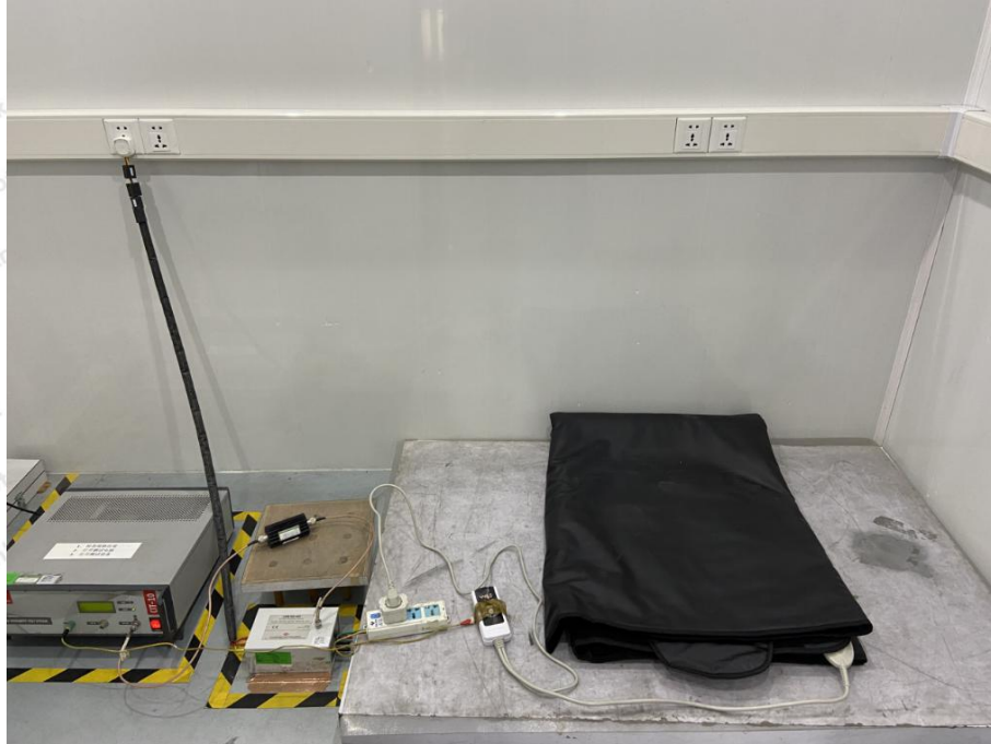
Photo of Injected currents susceptibility Test
