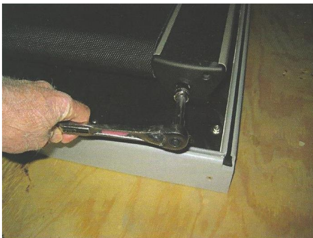
Figur 16. Justering af sporing (Tracking)
