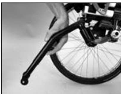
Fig. 41 Juster anti-tip sikringen
