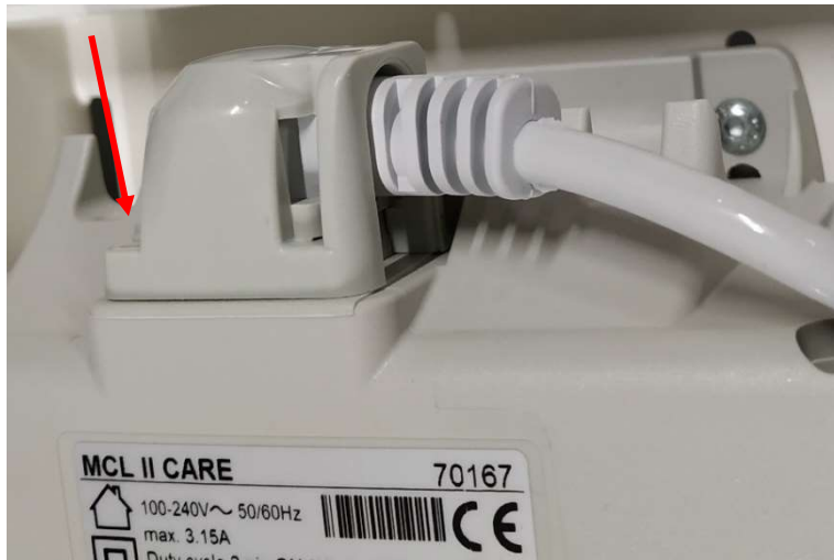
Image 53. Detachment of power cords' locking part
