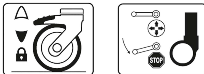
Image 10. Using brakes, individual and dual locking wheels
