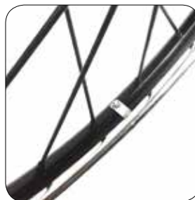
XL090 Handrim remove excess mounting tab
