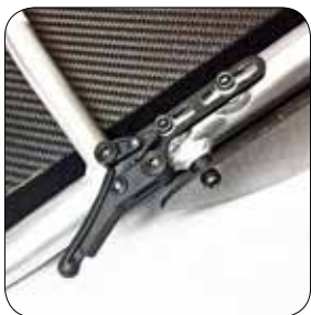
XD035 Brakes compact scissor with lightweight fixing
