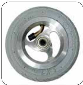
XC100 Castor wheel 5" pneumatic aluminium centre
