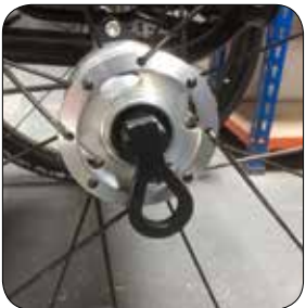
XK240 Wheel quad release axle nut (pair)
